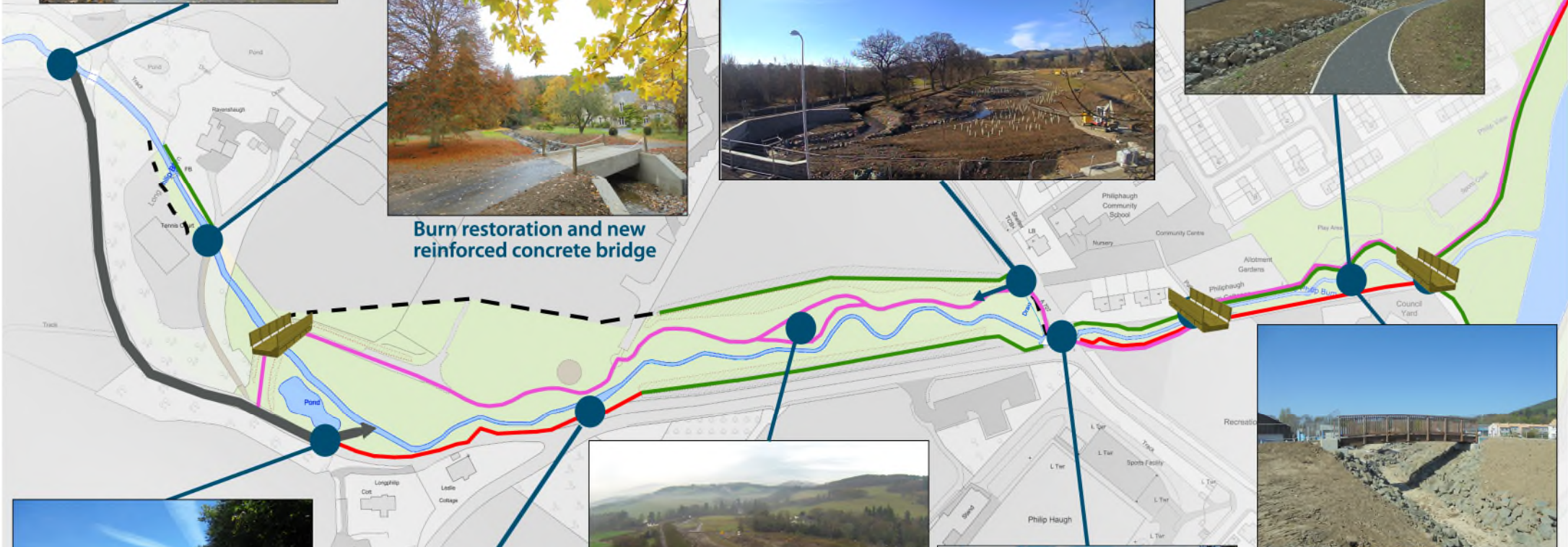
3 new Ekki timber footbridges raised above the 1 in 200 years flood level. Can remain open during high flow events
